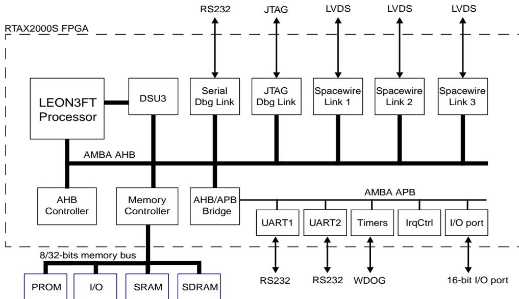
Figure 1. LEON3-FT-RTAX block diagram
