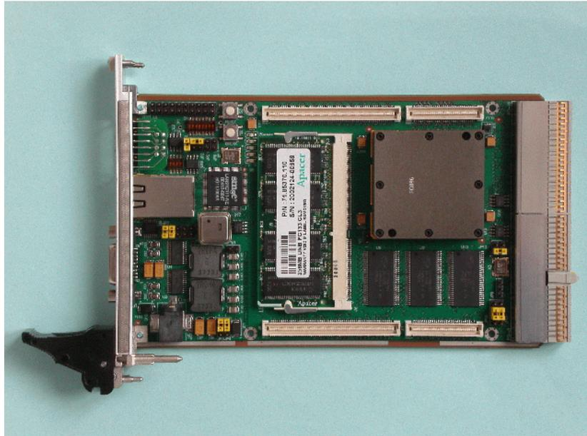
Figure 3. GR-CPCI-RTAX Development board (Pender, 2005)
