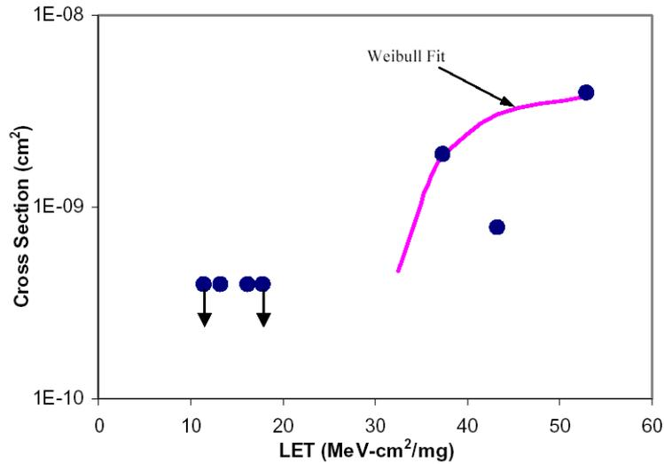
Figure 6. RTAX2000S RAM cell cross-section measurement (J.Wang - Actel, 2004)
