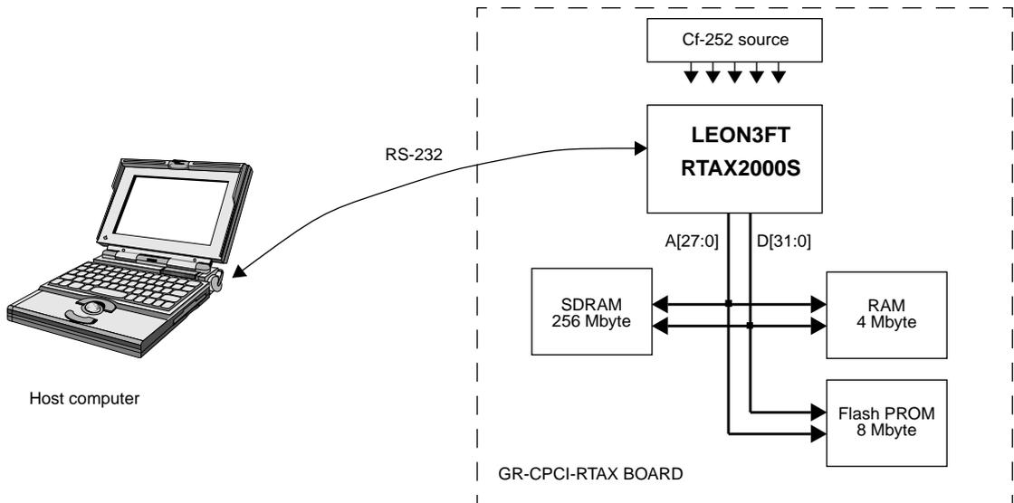
Figure 2. Test system architecture
