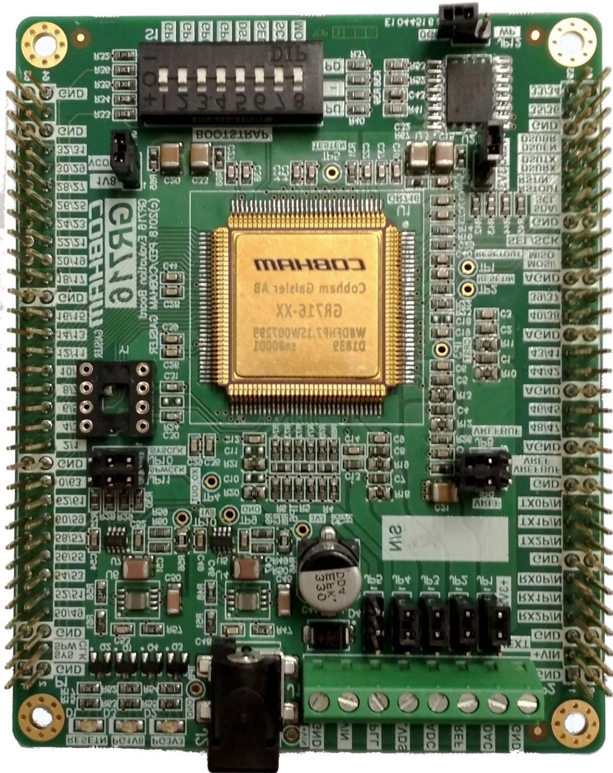
Figure 6-3 PCB Top View (Photo)
